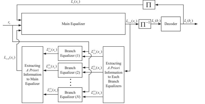
Fig. 3: Turbo Self-Iterating Soft Equalization Scheme.
