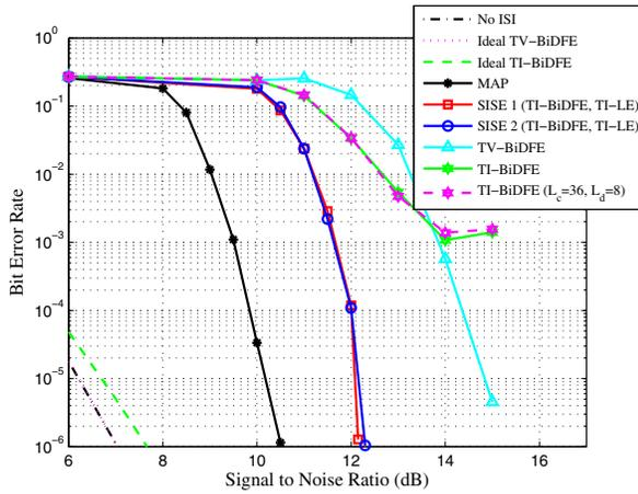
Fig. 6: BER Curves on the Channel  $h_3$  after 20 outer iterations.
