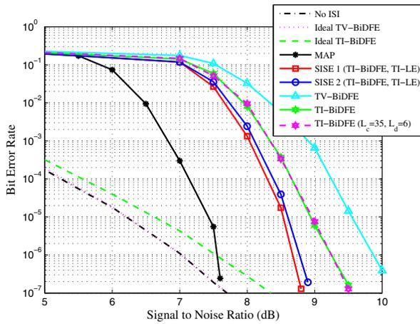
Fig. 5: BER Curves on the Channel  $h_2$  after 20 outer iterations.
