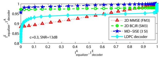
Fig. 5. EXIT chart for the different 2-D equalizers and the LDPC decoder.
