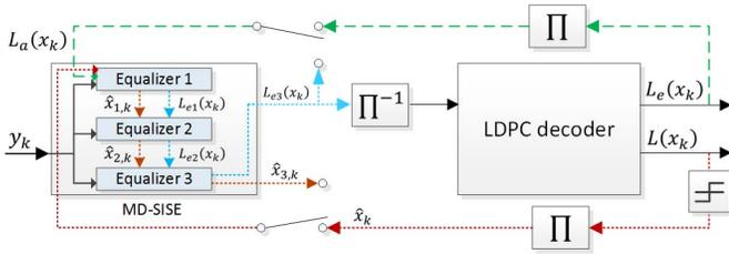
Fig. 2. MD-SISE based turbo equalizer.
