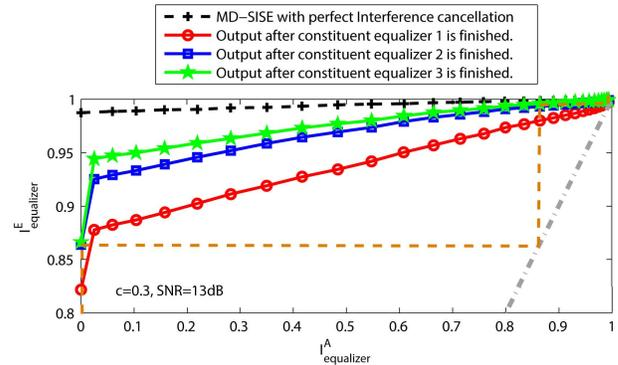
Fig. 4. Output versus input MI curves through SIs in MD-SISE.
