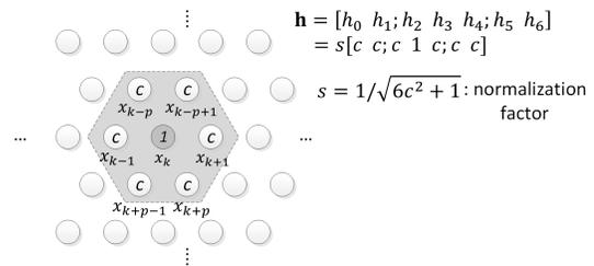
Fig. 1. 2-D array of data symbols, the ISI mask and the channel matrix.
