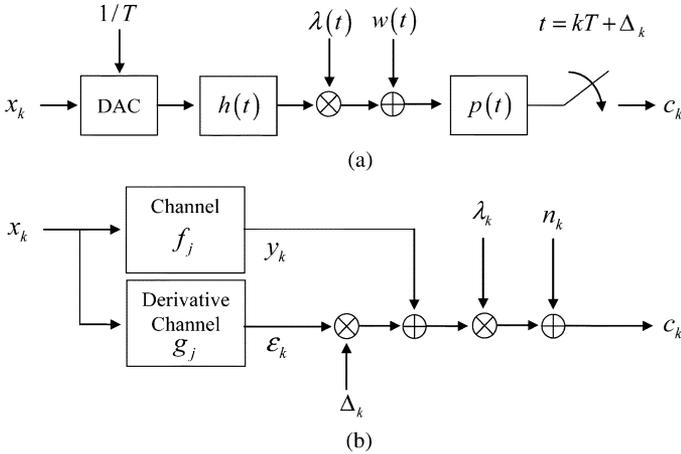
Fig. 1. Block diagrams of channel models. (a) Continuous-time channel model (b) Discrete-time channel model.
