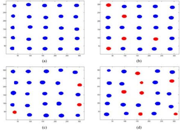
**Fig. 1: Sample magnetization waveforms generated under different noise environments: the red dots represent erroneously magnetized islands. Lithography jitter/SFD variation: (a) L/L (b) L/H (c) H/L (d) H/H**
